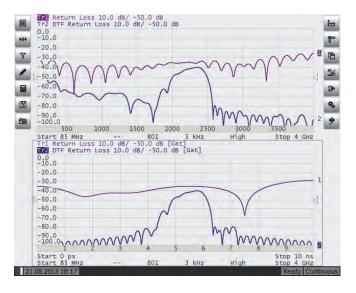
This function mathematically removes unwanted responses in the time domain, which allows the user to obtain frequency response without influence from the fixture elements. The function applies reverse transformation back to frequency domain after cutting out the user-defined span in time domain.
