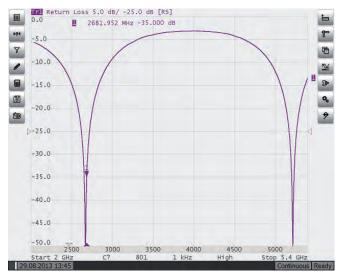
CMT 1-port VNAs can measure return loss as low as 35 dB, across the full frequency range of each instrument. Consult the specifications of each instrument for more detail.
