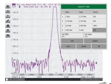
1-port VNAs (cable and antenna analyzers) have a large frequency range with the option of frequency scan segmentation. Among other benefits, this allows the user an opportunity to use the VNA, to realize the maximum dynamic range while maintaining high measurement speed.
