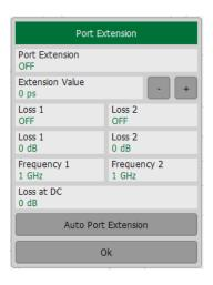
Port Extension is a feature that allows for moving the calibration reference plane of the port by specifying the electrical delay to the new reference plane position. Additionally, it is possible to account for loss in the extended port.
