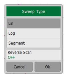
**Sweep type**: Linear frequency sweep, logarithmic frequency sweep, and segment frequency sweep.
