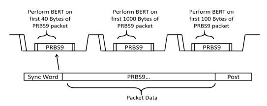
Figure 5 BER test capabilities with received HS data packets
