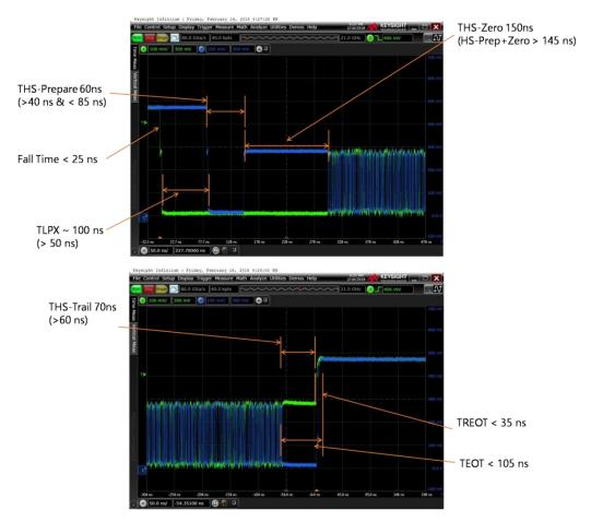
Figure 4 Typical SV4D DPTX HS Entry and HS Exit waveforms at 2.5 Gbps
