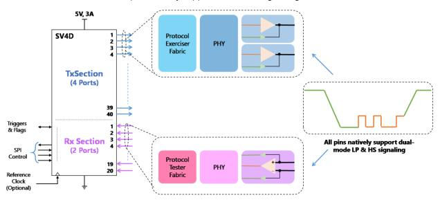
Figure 1 High level block diagram of the SV4D MIPI Test Module
