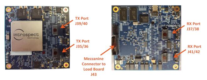
Figure 7 Connectors on top and bottom of the SV4D board
