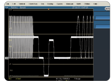
► Video Design. Illustration of triggering on an analog HDTV tri-level sync signal and examining horizontal blanking interval.
