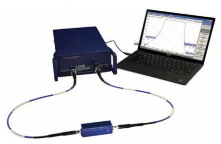
Cobalt VNAs have more than 162 dB dynamic range at 1 Hz IFBW, which allows them to maintain a wide measurement range at high measurement speeds. Measurement of all S-parameters of a BTS filter with full two-port and 801 measurement points with 1 MHz IFBW takes only 17.5ms while maintaining a measurement range of over 100 dB. This time is almost completely determined by the IFBW of the VNA. This measurement speed allows for real time tuning of high isolation BTS filters.
