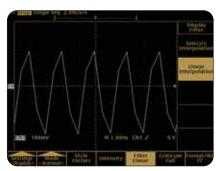
Even with 2 GS/s sample rate, which exceeds the Nyquist requirement of 2X oversampling, this 500 MHz oscilloscope with linear interpolation does not provide accurate reconstruction of the same 500 MHz sine wave.
