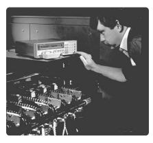
The 4263B LCR meter is designed for automated applications.
