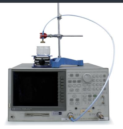
LimeSAR kit has been developed by MVG to measure material dielectric properties (complex permittivity and conductivity).
