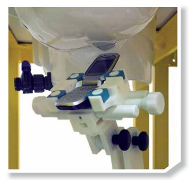
The handset positioning system developed by SATIMO complies with the standards in force for SAR and HAC measurements.
