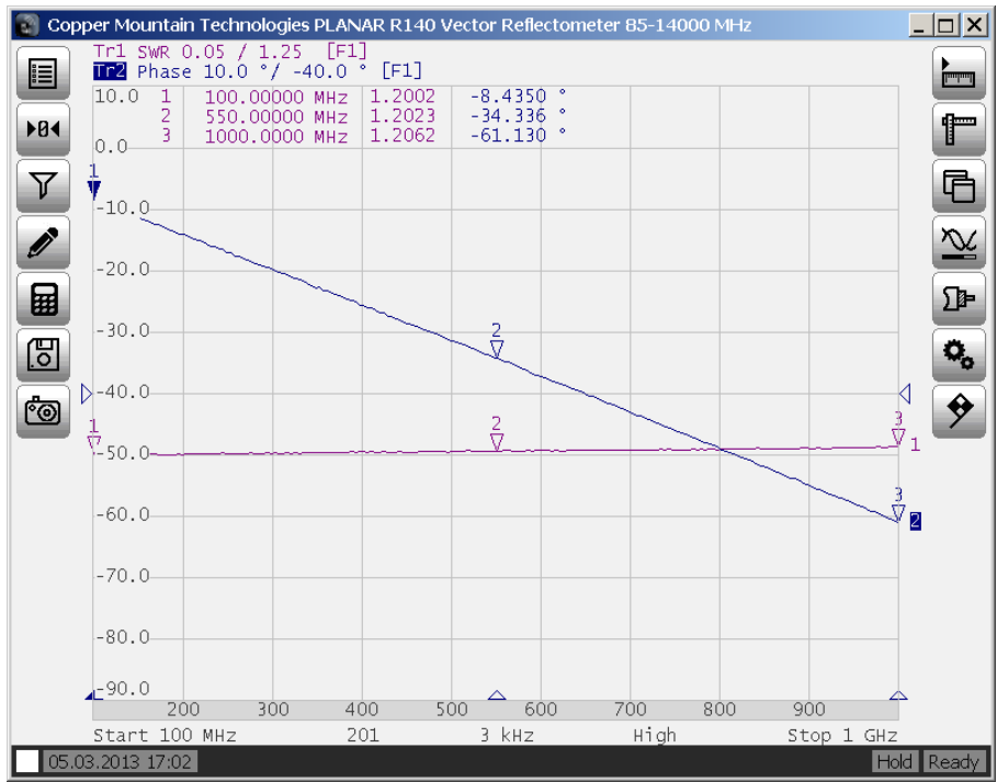
Figure 3.1 SWR and reflection coefficient phase measurement example
