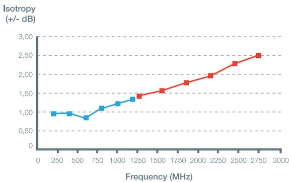
100 KHz - 3 GHz Axial Isotropy with vertical polarization
