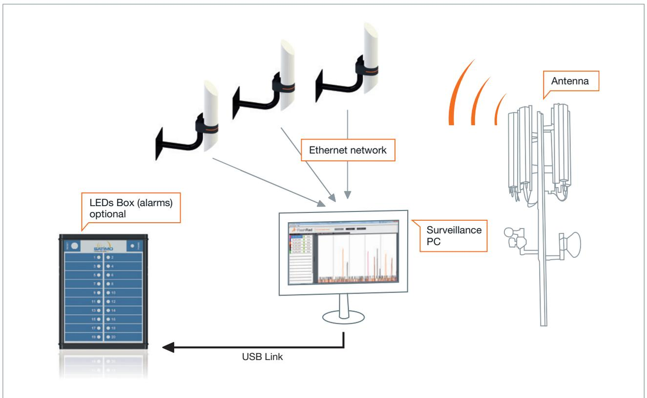
FlashRads are connected to a PC via Ethernet. Continuous EMF level measurements are sent to the PC where the FlashRad monitoring system software collects and displays the incoming data. If the FlashRads detect excessive RF levels, a signal is sent to the PC indicating which monitor is detecting the overexposed area. The technician can then take action. Note that each monitor can be stopped or started as necessary.
