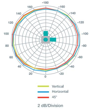
100 KHz - 3 GHz probe sensitivity without amplifier
