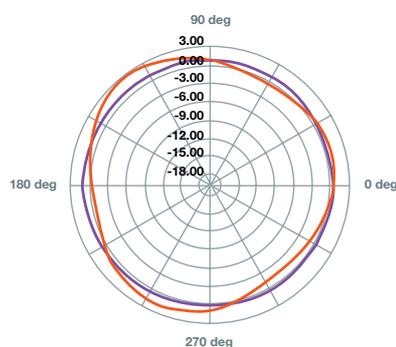
700 MHz - 6 GHz probe sensitivity
