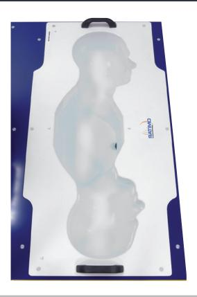
The SAM phantom (Specific Anthropomorphic Mannequin) developed by SATIMO is produced in accordance with the 3D-CAD files as specified in the standards and is delivered with a compliance certificate. It has been designed to fit the COMOSAR phantom tables and is delivered with a plastic cover to prevent liquid evaporation.
