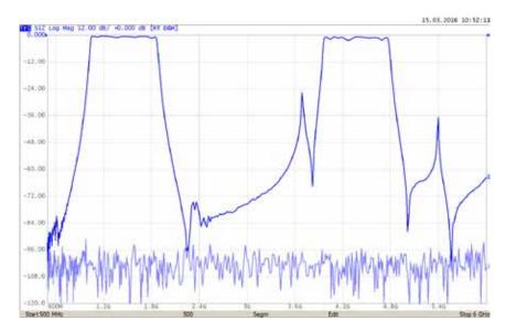
The 145 dB dynamic range of Cobalt VNAs combined with high measurement speed per point allows measurement of SAW filters' S-parameters with full 2-port calibration and 1601 measurement points in less than 32 ms while still maintaining more than 100 dB measurement range (IFBW at 1 MHz). This measurement speed corresponds to the performance of the most advanced handlers used for automatic verification of mass-produced SAW filters.
