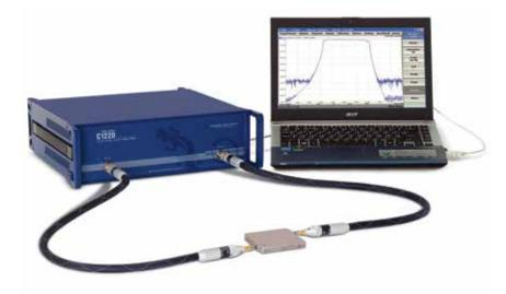
Cobalt 20 GHz VNAs have 145 dB dynamic range at 1 Hz IFBW, which allows them to maintain a wide measurement range at high measurement speeds. Measurement of all S-parameters of a BTS filter with full two-port and 801 measurement points with 1 MHz IFBW takes only 17.5ms while maintaining a measurement range of over 100 dB. This time is almost completely determined by the IFBW of the VNA. This measurement speed allows for real time tuning of high isolation BTS filters.
