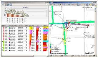
Additional analysis: PCI can be batch modify to simulate the result and compare the result after modification. This function can help engineer to understand the result will be before actually modify the PCI.
