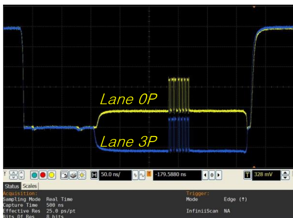
SV3C-DPTX programming a positive CM voltage for Lane 0 and a negative CM voltage for Lane 3
