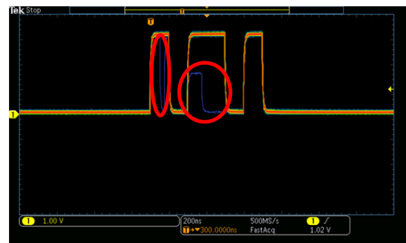
Figure 3: FastAcq capture of signal anomalies
