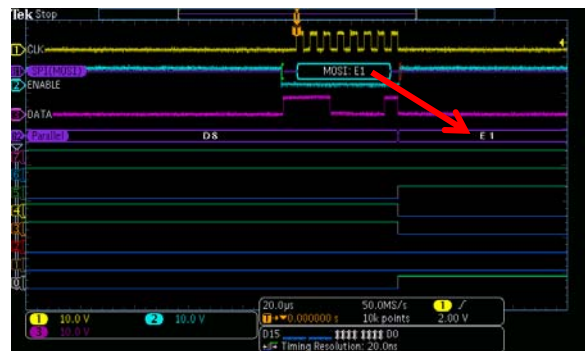
Figure 10: Digital channels and an 8-bit parallel bus added to the display.
