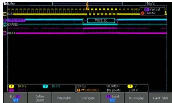
Figure 9: Automatic decode of the SPI serial bus.
