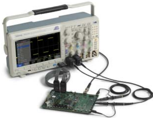
Figure 18: Using the integrated arbitrary / function generator as a source.
