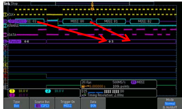
Figure 11: Mixed signal display stabilized with serial trigger capturing B0 hex data packet.
