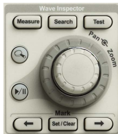
Figure 5: Front panel Wave Inspector controls
