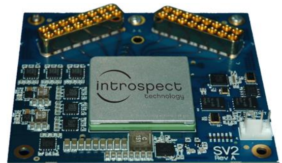
SV2D Direct Attach SerDes Test Module bolts onto any test card and offers full-featured 8 Lane, 28 Gbps production test coverage
