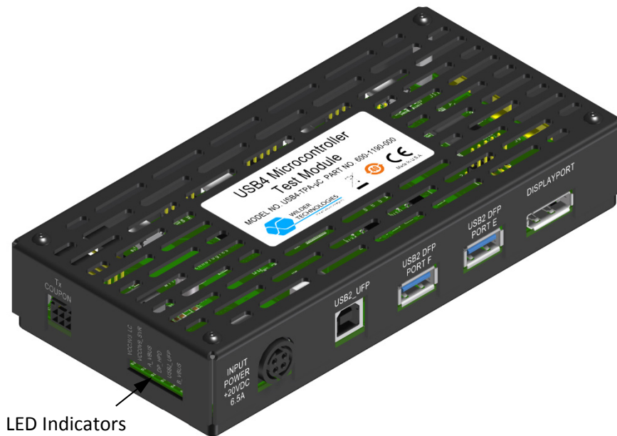
Figure 7. USB4 Microcontroller LED Status Indicators
