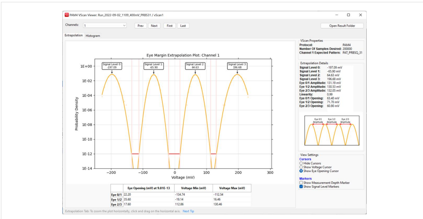
Figure 4: SV2C-PAM4 receiver measurement of vertical eye opening and linearity as viewed in the Introspect ESP Software
